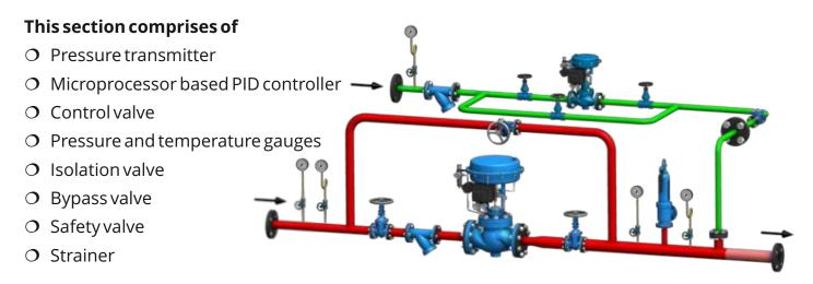
Pressure transmitter measures steam pressure at inlet/outlet and gives corresponding signal to PID controller. Depending on the deviation of existing pressure from required set value, controller gives command to modulate control valve and thus inlet/outlet steam pressure is maintained.
